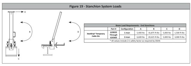
Note: The maximum single span length when using stanchions is 60', see Figure 20. The overall system length can be increased by using intermediate stanchions to create multiple spans in at most 60' increments. For multiple spans two FallTech SteelGrip® Coil Energy Absorbers must be used, see Figure 21.
