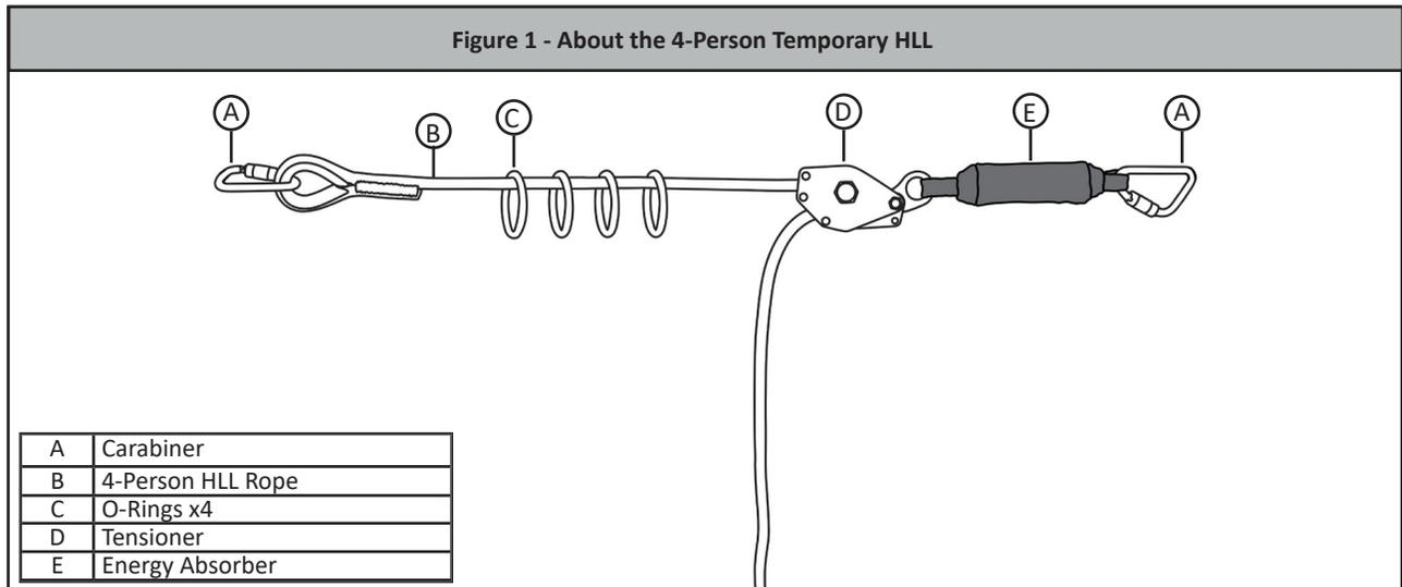
When properly tensioned, the lifeline will react to a fall event of up to four workers by combining the energy absorbing properties of the lifeline energy absorber, the lifeline, and the worker's personal energy absorber. During a fall event, the stretch of the lifeline and the expansion of the user's PFAS will result in reduced forces to the anchor and to the user's body.
