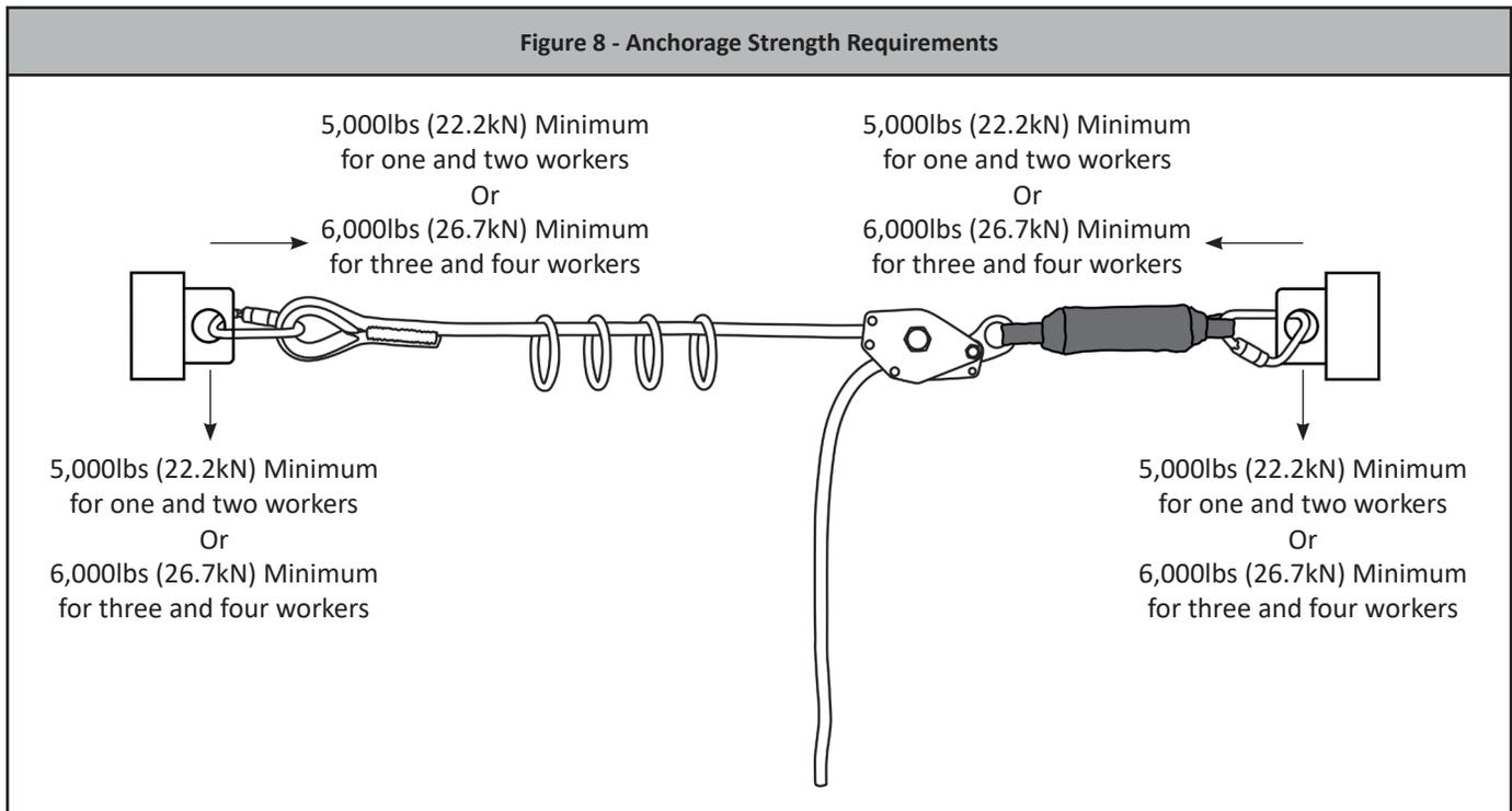
**Step 1:** Determine the location of the end anchorages and, in accordance with Section 3.2, evaluate their strength. Determine the span length of the system and determine the minimum required clearance for safe use in accordance with Section 2.7.
