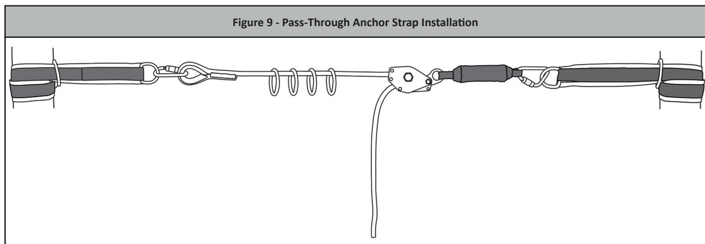
**Step 3:** Secure the HLL system to the anchorage connectors with the provided end attachment carabiners.
