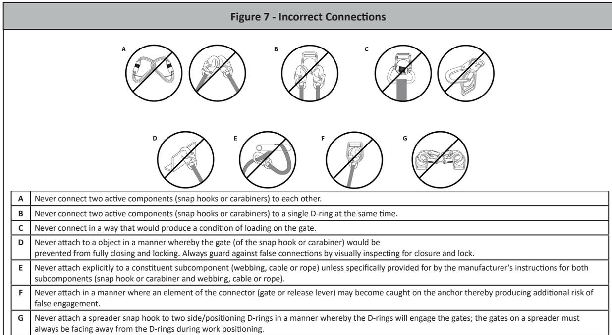
**3.4 Connectors:** Only use self-locking snap hooks, rebar hooks, and carabiners with this equipment. Only use connectors that are suitable to each application. Ensure all connections are compatible in size, shape and strength. Do not use equipment that is not compatible. Visually ensure all connectors close and lock completely. Connectors (snap hooks, rebar hooks, and carabiners) are designed for use only as specified in this manual.
