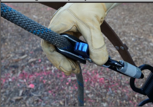
Figure 15: Rope Adjuster Release
