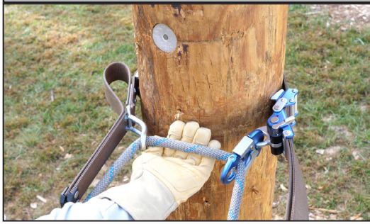
Figure 13: Acceptable Inner Rope Orientation
