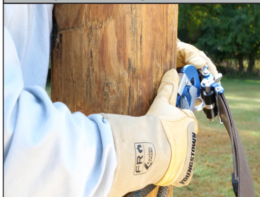
Figure 6: Connecting Device to Pole
