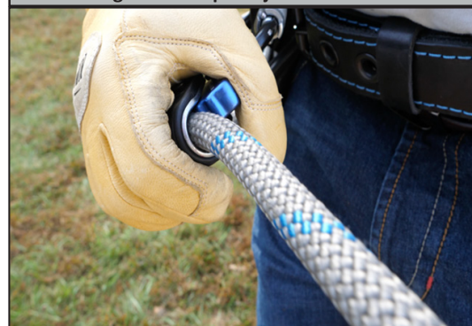
Figure 16: Rope Adjuster Release
