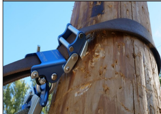
Figure 10: Vertical Cleat Engagement
