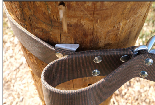
Figure 12: Fixed Web Strap Side Proper Adjustment
