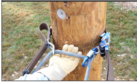
Figure 13: Acceptable Inner Rope Orientation
