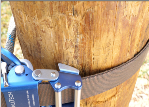
Figure 9: Horizontal Cleat Smooth Climbing
