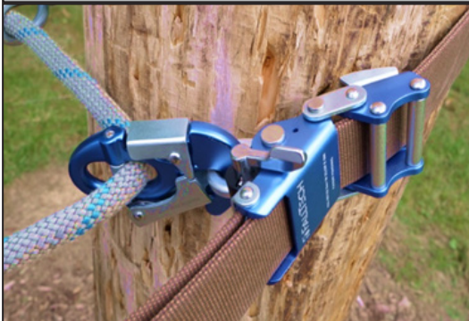
Figure 11: Strap Adjuster Side Proper Adjustment
