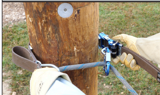
Figure 8: Moving Strap Adjuster Away from Pole
