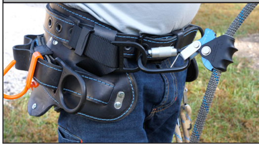
Figure 4: Connecting Device to Body Belt
