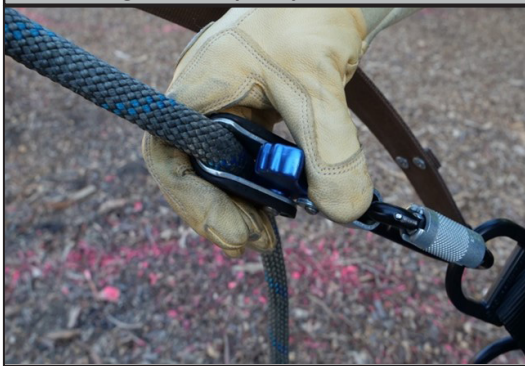
Figure 15: Rope Adjuster Release
