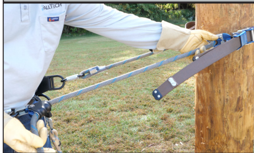
Figure 14: Moving Rope Adjuster Towards Pole
