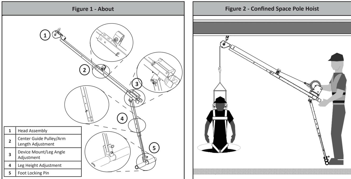
**2.2 Purpose:** The FallTech Confined Space Pole Hoist is designed to work as part of a system to raise or lower a person or material to work in a confined space for entry, retrieval, fall arrest applications, and material handling using a winch or Self Retracting Lifeline - Retrieval (SRL-R). The Pole Hoist is used along with an overhead anchor point for confined space openings such as manholes, sewer openings, and tank hatches.
