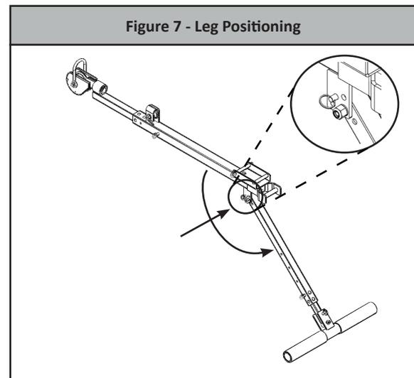
**4.1.4** Remove the Top Arm detent pin to adjust the length of the arm. Based on which detent pin hole is used, there is a 6" adjustment in which the arm can be lengthened.
