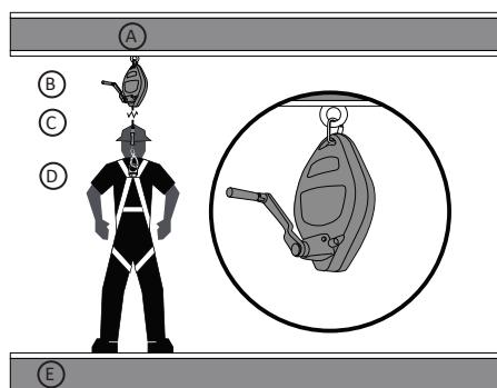
**Figure 4 - SRL-R Overhead Anchorage**
