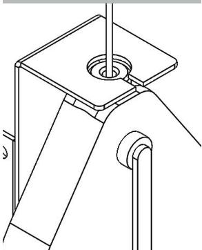
1. Remove the bolt and washer from the bracket and fold down the lower flap as shown in Figure 6.
