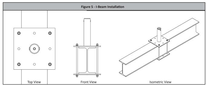
5.7 Weld-On Installation: FallTech® requires that the following steps be taken during the installation of this Post Anchor.
