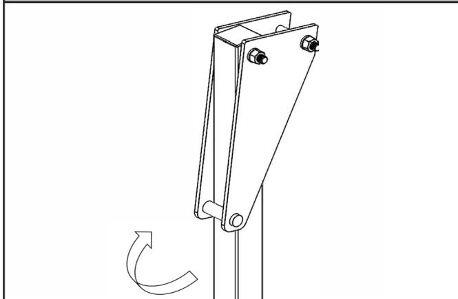
Figure 3- Large Offset Bolt-On Stanchion Assembled
