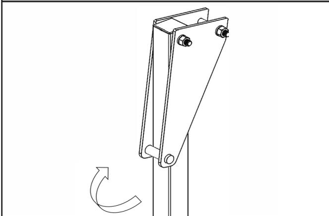
Figure 3- Large Offset Bolt-On Stanchion Assembled
