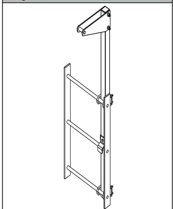
**5.2.2** If installing the Ladder Stanchion Anchor to the rear of the ladder rungs, it is necessary to reinstall the Bent Center Mount in the required orientation with the included 3/8" diameter bolt, washer, lock washer, and nut; torque to 15 ft-lbs; see Figure 8.
