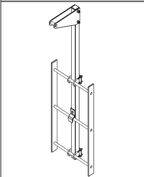
Figure 7 - Bolt-On Stanchion Side Mounted Rear
