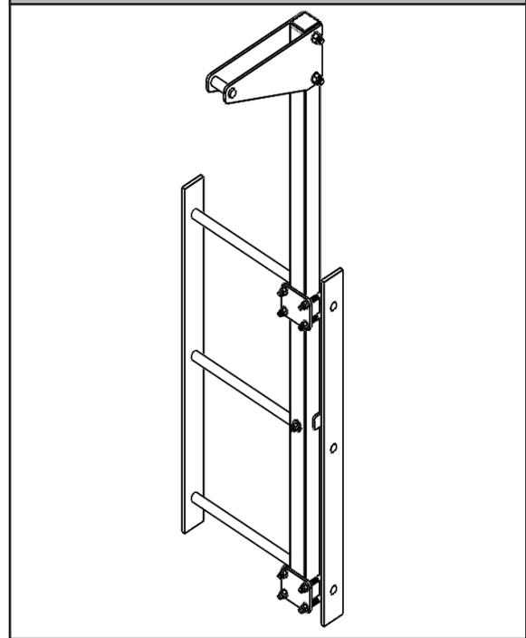
Figure 6 - Bolt-On Stanchion Center Mounted Rear
