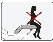
Do not sit or put unnecessary amounts of pressure on the leg section of the table when it is in tilt position of any level. This can damage or destroy the tilt mechanism and cause harm or bodily injury to persons. The tilt mechanism is intended solely to be used when a client is properly seated or laying on the table top. Damage caused in this manner may void the warranty.
