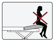
Do not sit or put unnecessary amounts of pressure on the back section of the table when it is in tilt position of any level. This can damage or destroy the tilt mechanism and cause harm or bodily injury to persons. The tilt mechanism is intended solely to be used when a client is properly seated or laying on the table top. Damage caused in this manner may void the warranty.
