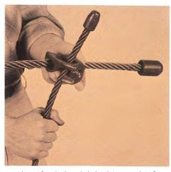
1. Insert ferrule-tipped choker into rope slot of hook so it projects 12" to 18" beyond hook - this is important! Then, rotate or turn the rope 90° toward vertical axis of hook.
