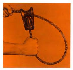
**3.** Line tension maintains positive connection without locking pins or keys.
