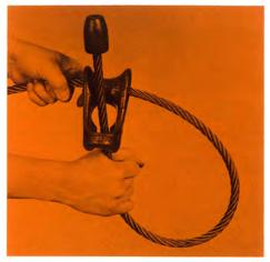
1. Insert ferrule end of rope through large keyhole opening of choker hook.
