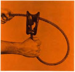
2. Pull choker rope down and into open slot of keyhole until ferrule seats in hook pocket.
