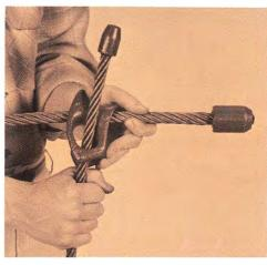
2. Pull choker straight down until choker ferrule is nesting in pocket of hook - this is a "snap-fit."
