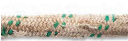
**THE REPAIR:** If you encounter a deeply abraded spot, where more than 50 percent of the strand is affected, you can re-splice the rope to repair it.
