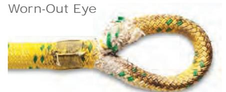
**THE REPAIR:** To repair a worn-out eye, you'll want to shorten, re-splice and reverse the rope. Proceed by putting the unused end into service.
