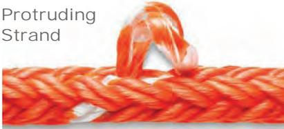
**THE REPAIR:** Work the strand back into the rope as soon as you notice it, by carefully tugging on adjacent strands until the excess is distributed evenly. A protruding strand in service could easily snag or break, causing further complications.
