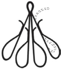
Each leg adjusts to accommodate any-sized load or lift-point arrangement. Lifts using less than four legs reduce the ratings proportionately.
