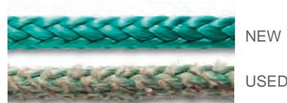
**THE REPAIR:** If the diameter is reduced by less than 10 percent, it is still able to remain in service. If the diameter reduction is 11–20 percent, downgrade the rope. Should the diameter reduction from new to used exceed 20 percent, retire the rope.
