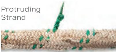
**THE REPAIR:** One to four strands spaced out by several feet can be removed and rewoven into the line with minimal impact on strength (less than 12 percent).
