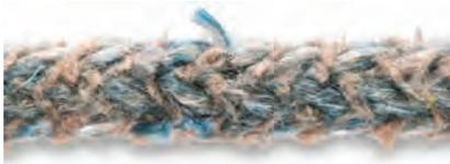
**THE REPAIR:** If possible, remove the affected section and re-splice with an end-for-end splice. If re-splicing is not possible, retire the rope. As a general rule, 12-strand ropes should be retired when more than three broken strands are visible.
