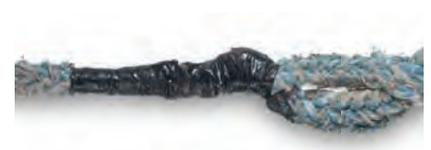
**THE REPAIR:** Re-splice the rope correctly.
