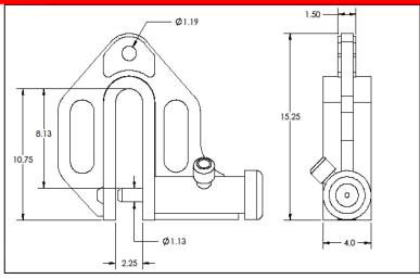
12 ton working load limit @ 4:1 design factor.
