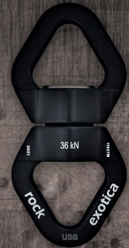
ROTATOR TRIANGLE (S1 L) Weight: 5.0 oz (143 gm) MBS: 36 kN Working load: 5 kN
