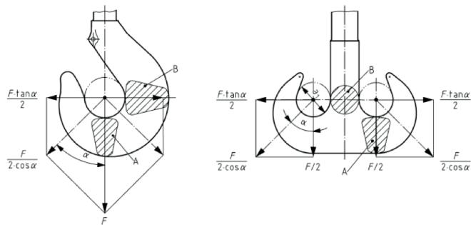
Skew loading shall be avoided by adjusting the rigging arrangement below the hook to allow the center of gravity of the load to line up with the centerline of the hook shank. The hook shall receive symmetrical vertical loads to minimize additional stress due to the bending of the hook shank.
