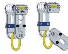
\* The Gated Trolley is tested to and meets the requirements of ANSI Z359.18 2017 for fall protection applications. Each trolley is rated 5000lb for this purpose.
