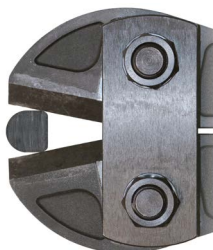
Design does not allow bolt cutters too get a good bite
