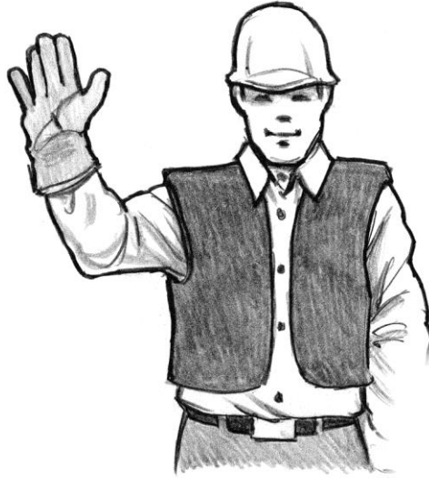
Figure 7-53 – Mainline Ahead Normal (Raise one arm)
