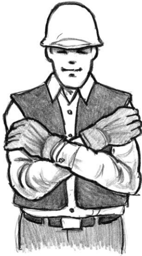
Figure 7-57 – Ahead On The Dropline (Cross arms in front)
