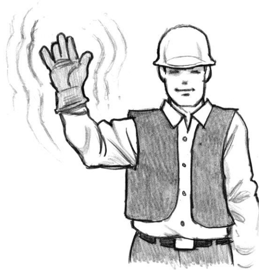
Figure 7-54 – Mainline Ahead (One arm raised, hand fluttering)
