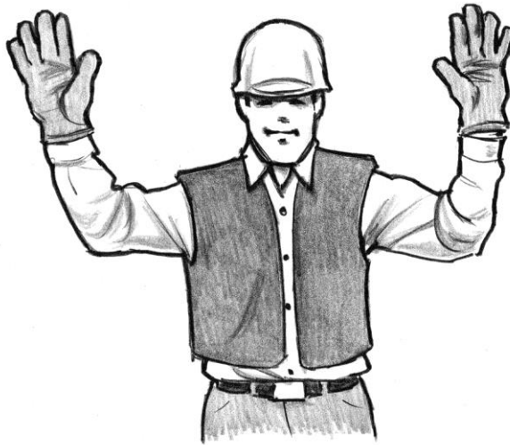
Figure 7-52 – Mainline Ahead Slow (Both arms raised)
