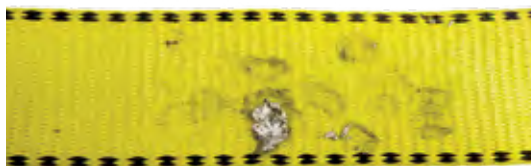
SLING WELD SPLATTERS
