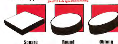
29-HP20 hole types for punching
