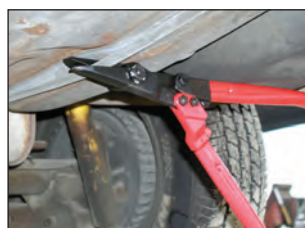
Cuts gas tank strap
