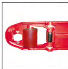
Entry/exit rollers and solid steel push rod
