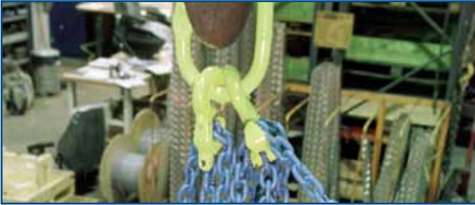
Fig. 7. "A three-leg, fully adjustable sling."
