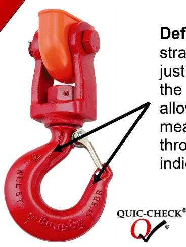
Deformation Indicators -- Two strategically placed marks, one just below the shank or eye and the other on the hook up, which allows for a QUIC-CHECK® measurement to determine if the throat opening has changed, thus indicating abuse or overload.
