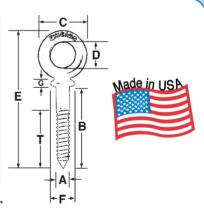
Screw eye bolts supplied with cone points - lag screw thread.
