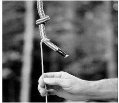
Tie a knot near the end of the rope and attach the string. As you pull on the other end of the climbing line, the knot will pass through the large ring, but not through the smaller ring, dislodging the Friction Saver. The Friction Saver can then be lowered. (If using spliced eyes on the end of your climbing line, you may attach a string to a key instead of using the knot).
