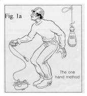
**1a.** Tie a slippery half hitch in line. This will provide a good finger hold.
