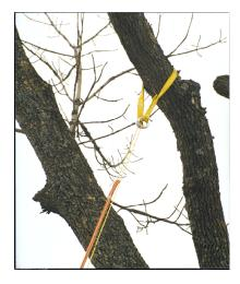
7. Attach throw line to climbing line eye using a clove hitch, if climbing line has no eye, attach using a series of 3-4 half hitches with a clove hitch tied 5-6" in from end of climbing line. Then simply pull the climbing line up and through the friction saver rings.
