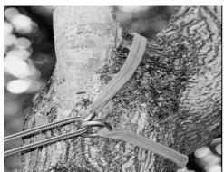
The Friction Saver offers consistent friction when working in different positions in the tree.
