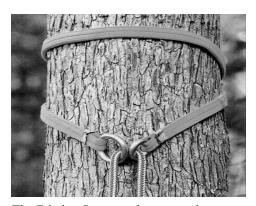
The Friction Saver can be wrapped on a stem where no natural crotch exists.
