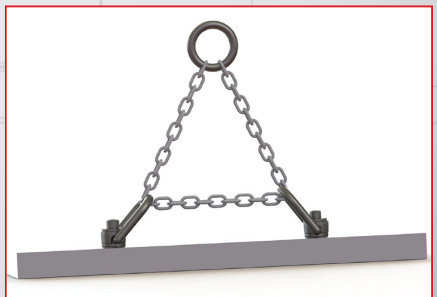
Unsafe Do Not Reeve
